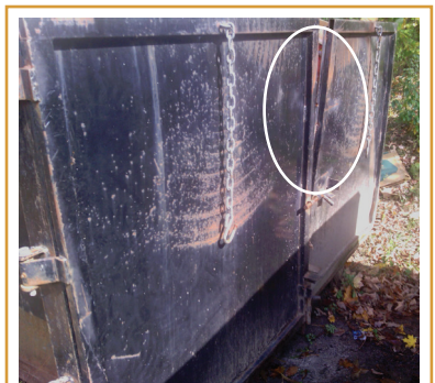
Competition's Boxes. Notice How The Doors Bow Out Because Doors Only Latch To Floor
